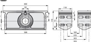
Caution for Upper and Bottom Brackets Recommended backlash between pin over-bosses and brackets / supports = 3 mm total (1.5 mm each side). It is recommended to fit M16 bolts/nuts, type 8.8 or better.
