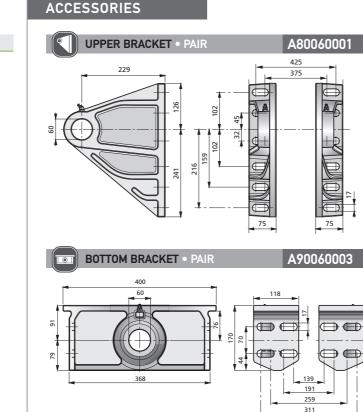
Caution for Upper and Bottom Brackets Recommended backlash between pin over-bosses and brackets / supports = 3 mm total (1.5 mm each side). It is recommended to fit M16 bolts/nuts, type 8.8 or better.
