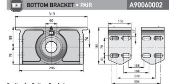
**Caution for Bottom Brackets** Recommended backlash between pin over-bosses and brackets / supports = 3 mm total (1.5 mm each side). It is recommended to fit M16 bolts/nuts, type 8.8 or better.
