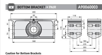
Recommended backlash between pin over-bosses and brackets / supports = 3 mm total (1.5 mm each side). It is recommended to fit M16 bolts/nuts, type 8.8 or better.
