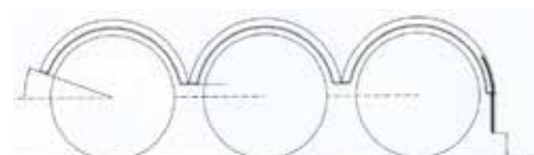
EXAMPLE 2. Non steered wheels distance between tyres less than 250 mm.
